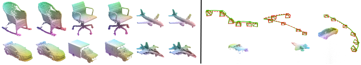
Figure 3.4: Canonicalization applications. Partial shape reconstruction (left section) shows pairs of GT (left) and predicted shapes (right). Pose estimation (right section) shows GT (green, solid) and predicted (red, dashed) camera pose based on regressed T-NOCS points. Points are colored by their T-NOCS location.
